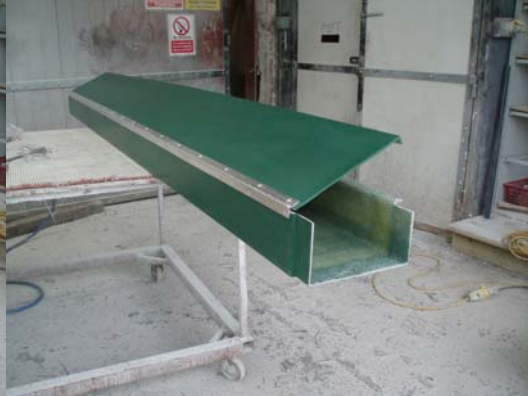
Each section has full-length hinged lid
