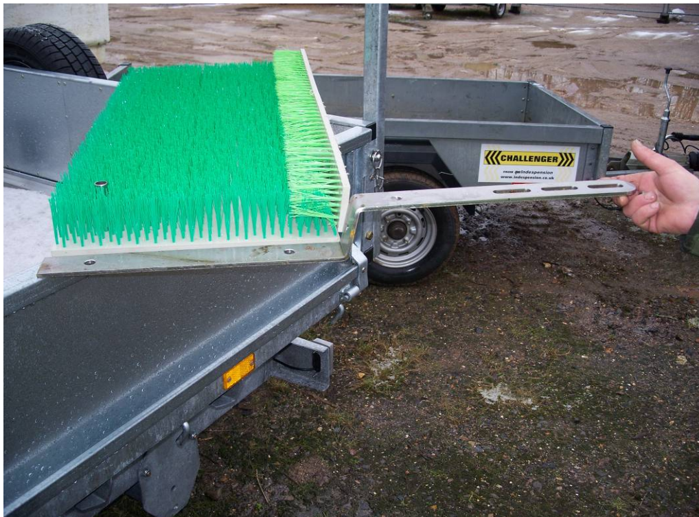
Figure 4.9: Pre-fabricated stainless steel bracket (showing stand-off)
