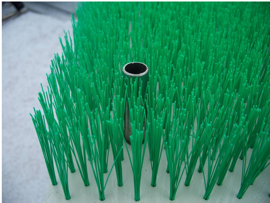
Figure 4.8: Bristle board with stainless steel spacer / nut
