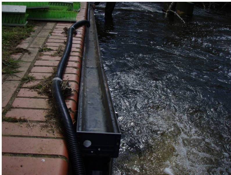
Figure 4.20: UPVC sectional drainage channel, fixed to side wall. (Hole for pumped water supply at near end, with pump tubing ready for fitting.)
