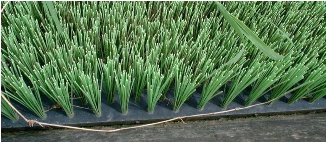
Figure 3.1: Bristle substrate with nylon bristles fixed to a polypropylene sheet
